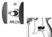
Set function selection switch to OFF. Lock trigger safety.
