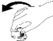
Turn pressure to lowest setting. Trigger gun to relieve pressure.
