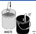
Remove siphon tube set from paint and place in flushing fluid. Use water for water base paint and mineral spirits for oil base paint.
