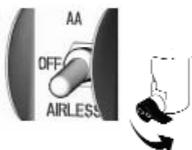
Plug in sprayer. Set function selection switch to AIRLESS. Turn prime valve horizontal.
