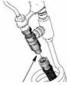
Connect blue fluid hose to fluid inlet fitting on gun fluid tube. Tighten securely.
