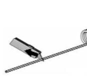
Cut air hose to length and couple to air connection on air/fluid supply hose.
