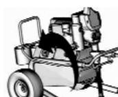
Tilt sprayer backward. Align end of direct immersion tube with bottom of pump.
