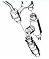
Attach fluid high pressure swivel and gun air regulator to gun.
