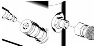
Attach air hose to sprayer air fitting and fluid hose to fluid fitting. Tighten securely.
