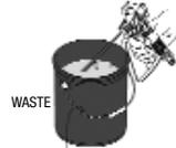
Hold gun against grounded metal flushing pail. Trigger gun and increase fluid pressure to 1/2. Flush 1 minute.
